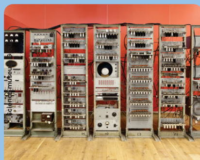
A replica of Baby, built by the Computer Conservation Society in 1998
